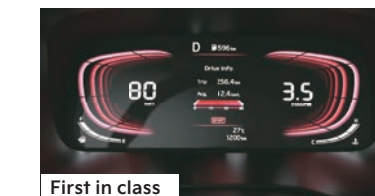
31.7 cm (12.5") Full Segment LCD Cluster with Advanced 10.6 cm (4.2") Color TFT MID
