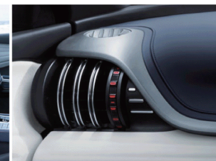
Dumbbell-style Air Conditioning Vents
